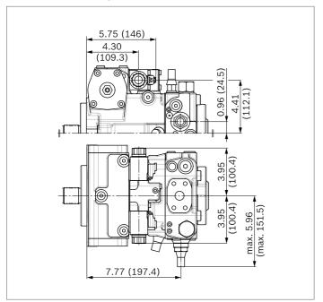
▼ DA..3 - Mechanically adjustable with position lever
